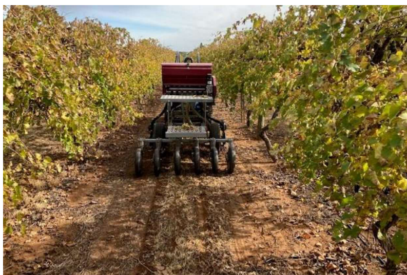
Figure 1. Seeding midrow cover crop with Taege seeder.
