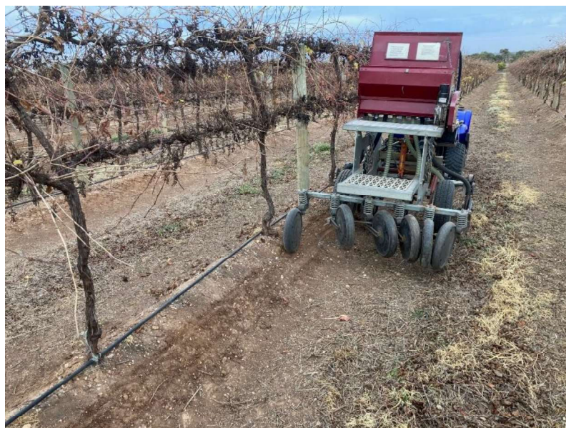
Figure 2. Seeding under-vine cover crop with Taege seeder
